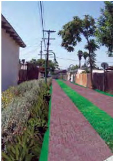
Rendering of the greened alley, featuring a “Hollywood driveway” with Grasscrete and permeable pavement, as well as drought-resistant landscaping and energy efficient streetlights.
