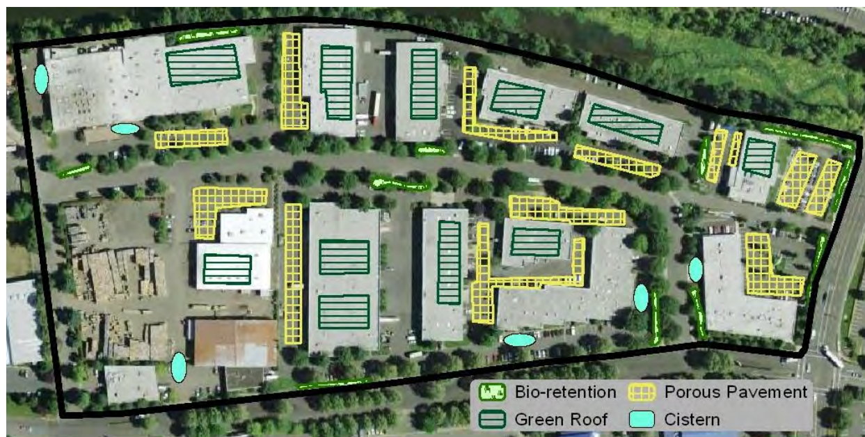
Figure 15. Actual Site and Onsite Control Measures (Portland, OR)
