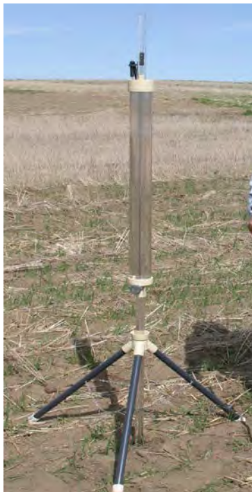
Figure C-3: Guelph Permeameter for Shallow Borehole Permeability
