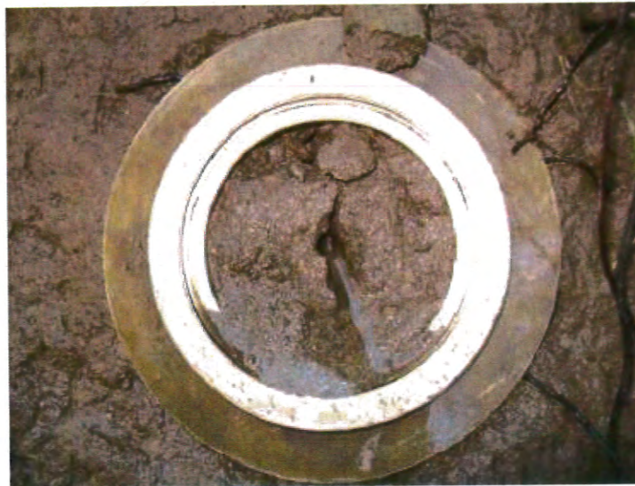
Hole created in cohesive bank material by jet impinging on surface
