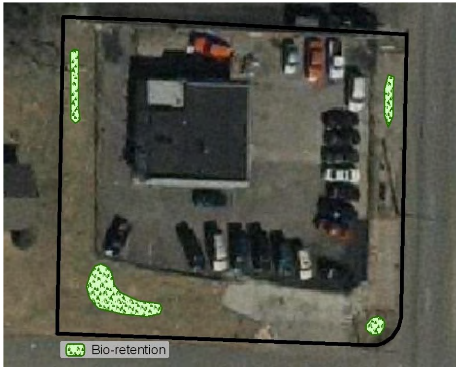
Figure 12. Actual Site and Onsite Control Measures (Charleston, WV)
