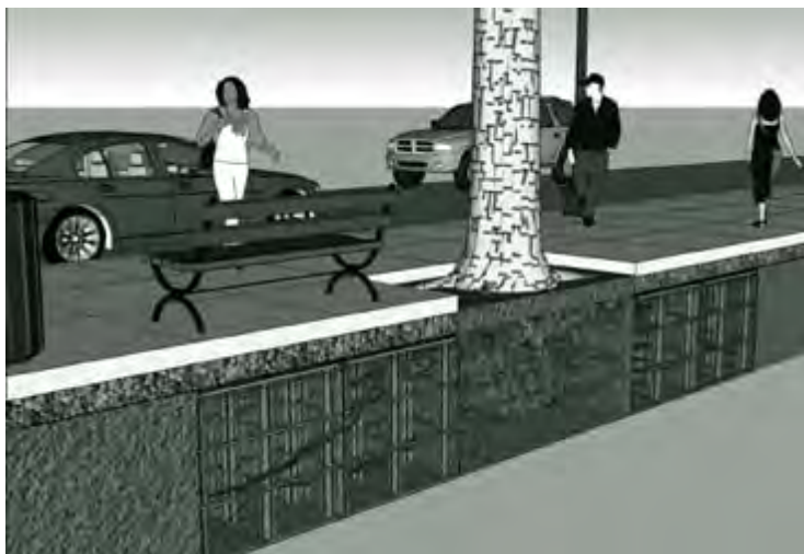
Figure 6. Silva cell structures support the sidewalk while providing root space for street trees (Source: Deep Root Partners, LP).
