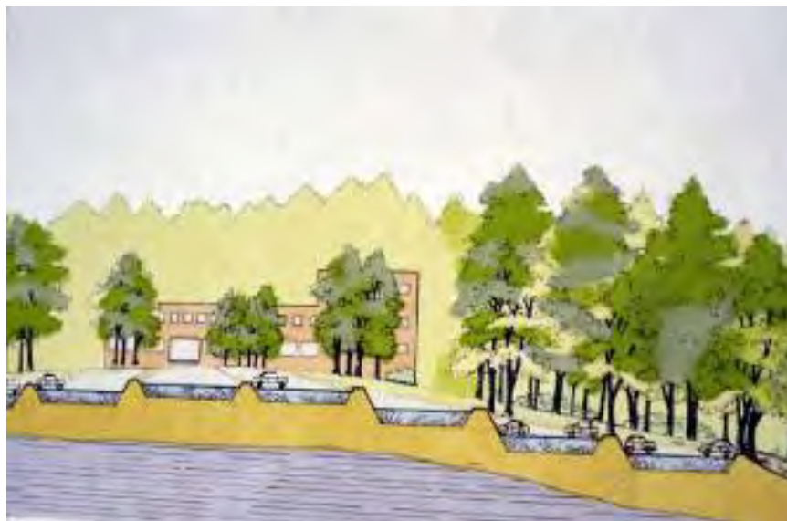
Figure 54. Design subsurface infiltration beds to “step” down a slope, maintaining level bed bottoms and earthen berms between beds.
